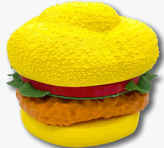
Assembly of color prints made using FDM
