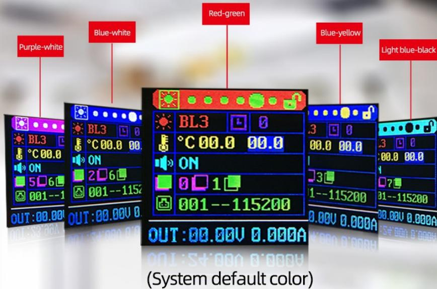
Short press the rotary encoder button, select the corresponding position, the corresponding number will be reversed, use the rotary encoder to switch the theme background color and foreground color
