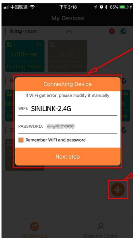
During the pairing process, the WiFi network must be 2.4G, and 5g network cannot be paired. (if your WiFi router 2.4G and 5g are network combined, please reconfigure the router, separate them, and select 2.4G network)
