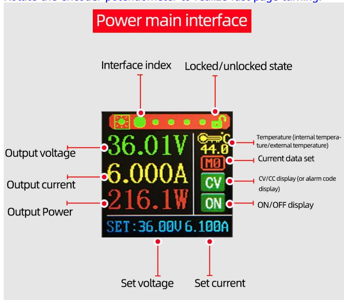
Short press the code potentiometer button to activate the parameter (voltage/current) to be set;
