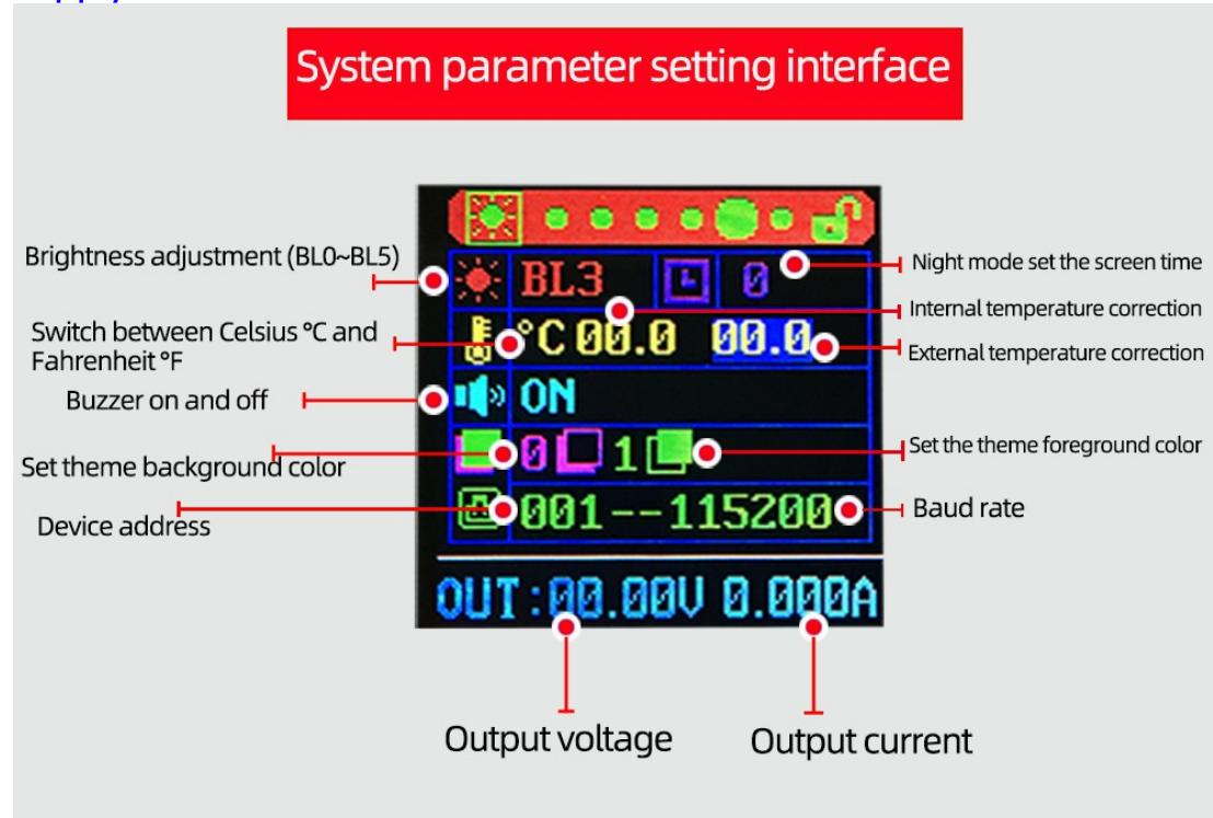
Short press the code potentiometer button to select/switch the parameter to be set. After selecting, the parameter will be reversed and set the parameter through the rotary encoder;
