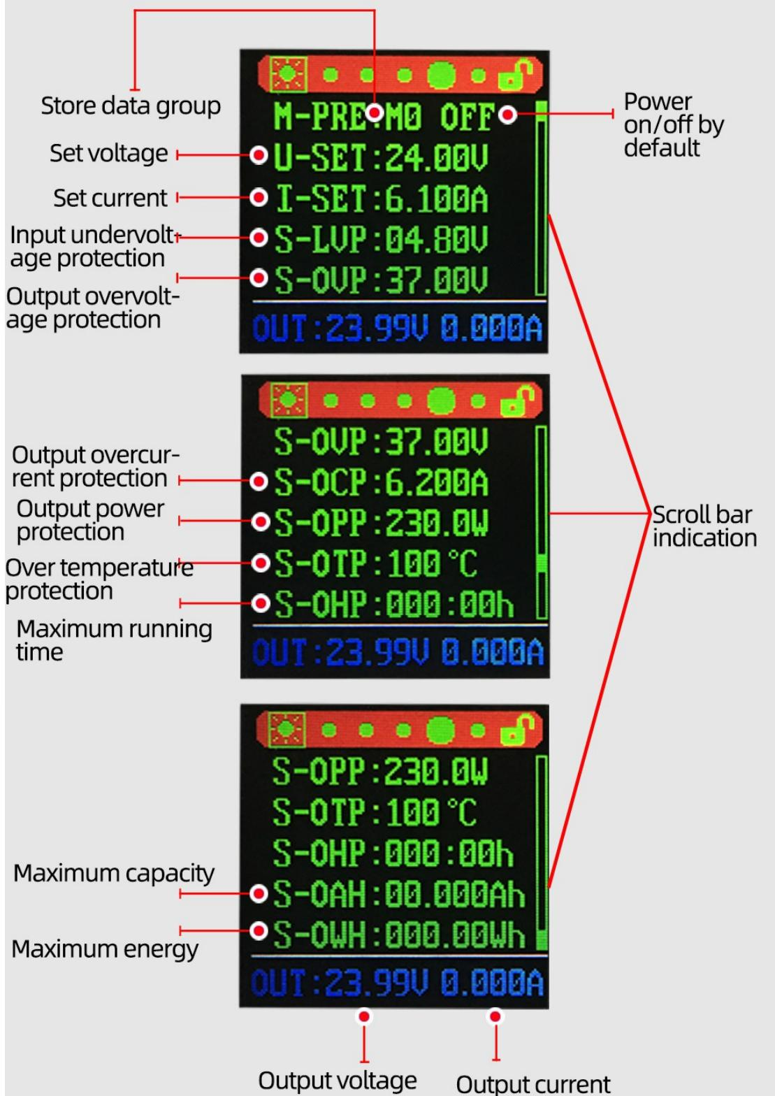
Short press the code potentiometer button to activate the parameter to be set;
