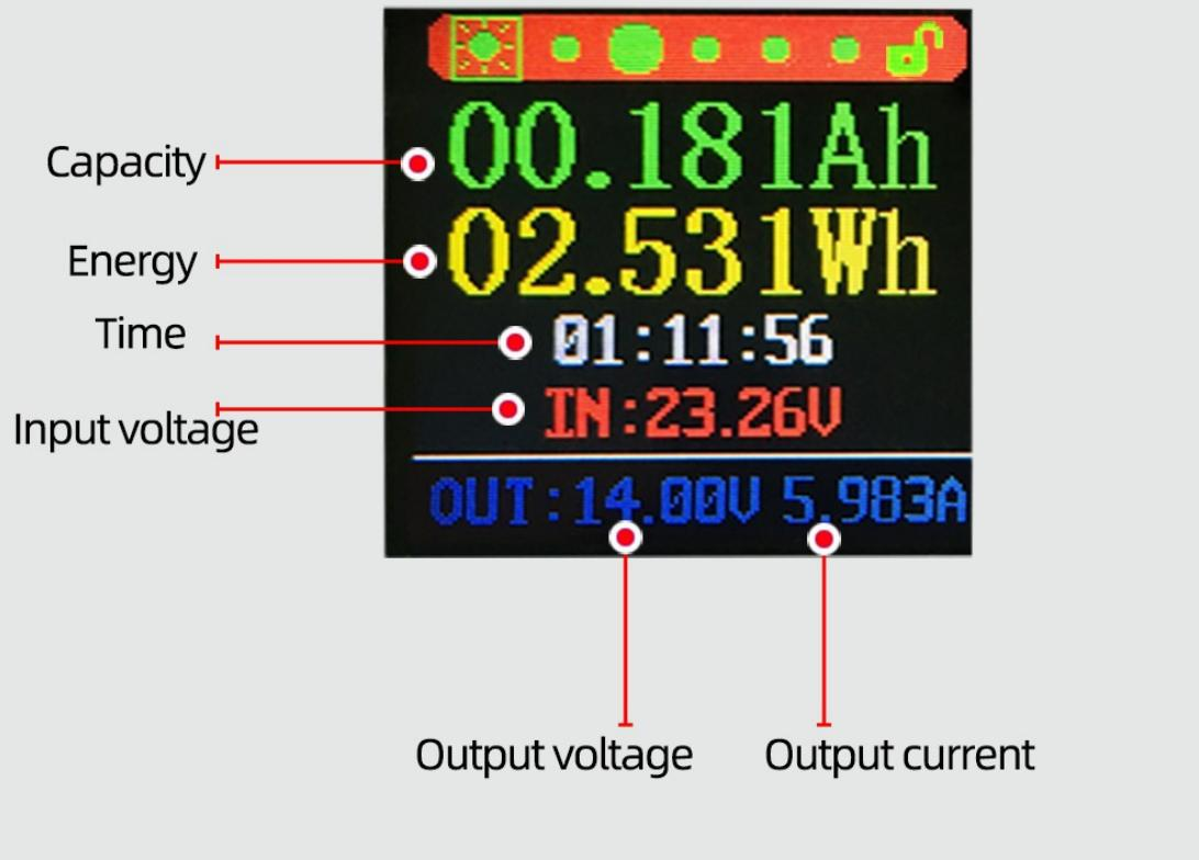
Short press the code potentiometer button, select all'capacity/energy/time', and the corresponding one will be displayed in reverse blue after all selections. Use the rotary encoder to switch the parameter to be cleared. After selecting, short press the code potentiometer button. Clear the corresponding parameter; after selecting, long press the code potentiometer button for 2 seconds or no key operation for more than 6 seconds will automatically exit.
