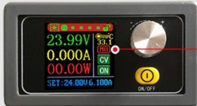
A total of 10 groups of data can be stored for M0-M9, which are saved to data group M0 by default, and M1/M2 data groups can be quickly recalled.
