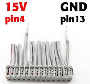
Figure 8.8.4 - Custom 13-pin wire harness for external DC supply
