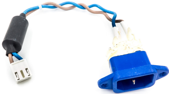
Figure 8.3.2 - Custom AC wiring harness for K.2. Add a resettable 3A circuit breaker in series for added protection (not pictured).
