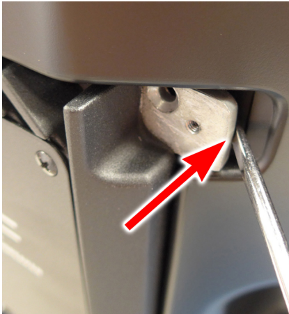
Figure 5.1.3 - Prying amplifier module away from enclosure.
