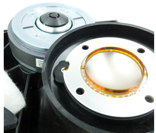
Figure 5.4.3 - Diaphragm removal with HF transducer still fastened to baffle
