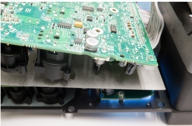
Figure 8.8.1 - Testing with a golden input/DSP board (verified)
