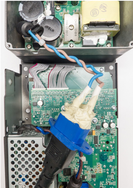
Figure 8.3.1 - Bypassing the AC line filter using a custom AC wiring harness
