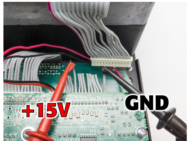
Figure 8.8.5 - Applying +15V using an external supply
