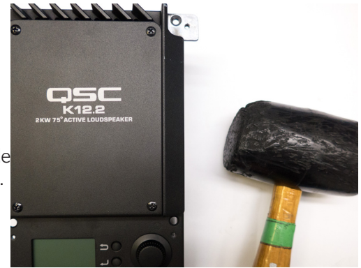
Figure 7.2.3 - Lightly applying force to the amplifier module to find intermittent connections.
