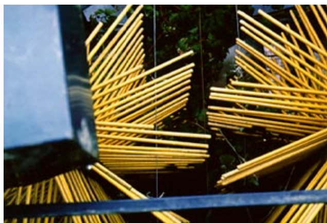
Top side view from the harvest machine, looking down on picking rods, which shake the fruit from the row.
